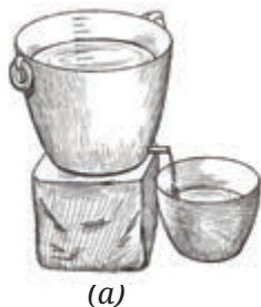
Fig. 8.2 A water clock (a) Water flowing out-type (b) Floating bowl-type
